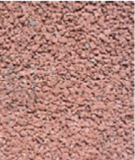
Colored Porous Asphalt
