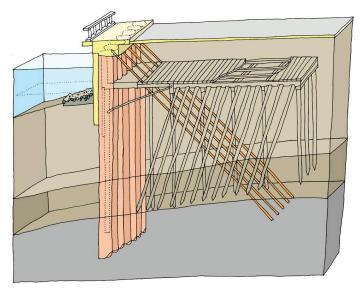
Braced soldier piles structure in cross-section (shown in orange)
