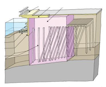
*Jet grouting structure in cross-section (as shown in purple)*
