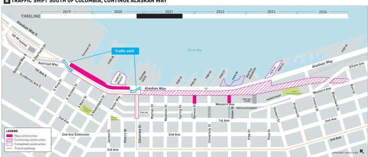
In fall 2020, traffic will shift to the new Alaskan Way, in the footprint of the former viaduct, from S King to Columbia streets. We will be continuing utility work on the new Alaskan Way north of Columbia. The removal of Pier 58 will be completed in early 2021.
