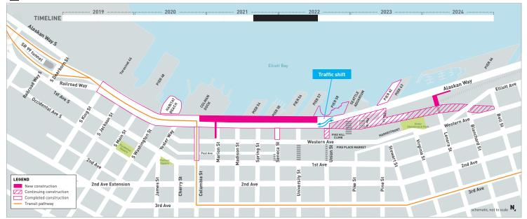
We will continue work on the elevated portion of Alaskan Way, which will become Elliott Way north of Pine Street. In fall 2021, traffic will shift to the new Alaskan Way, in the footprint of the former viaduct, from Columbia to Union streets. Construction of the Park Promenade between Columbia and Union streets will begin.
