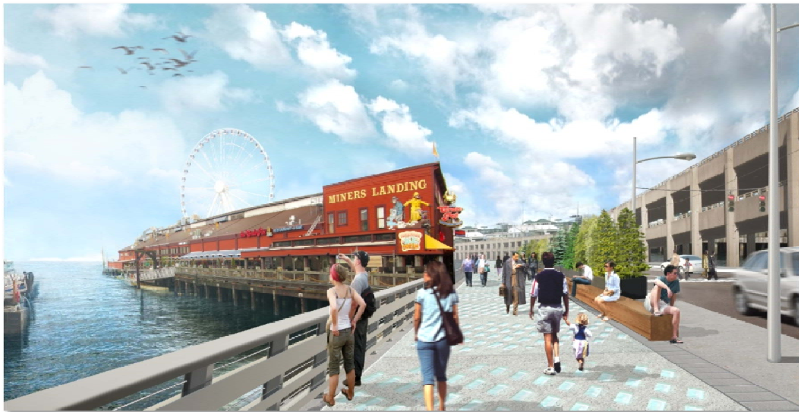
Rendering of the new sidewalk with light-penetrating surface to transmit light to the habitat below
